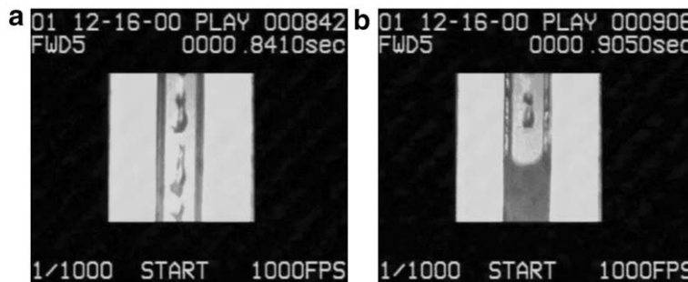
Fig. 3. Flow pattern downstream the ONB: (a) dryout, (b) single phase water flow.
